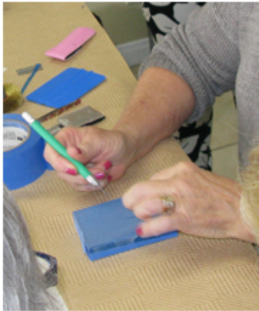
pulling off portions of the mask to do a light frosted sandblast layer.
